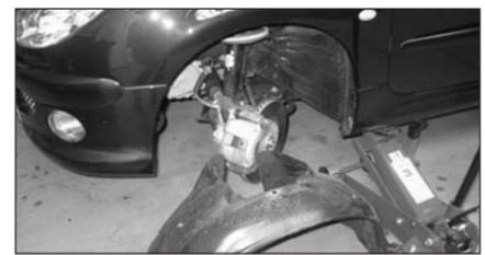
12. Taking the necessary safety precautions raise the front of the vehicle and support it with axle stands. Now remove the wheel and wheel arch liner from the vehicle as shown.
