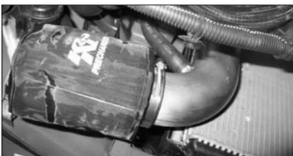
29. Fit the Drycharger over the filter as shown. **NOTE:** The Drycharger's water repellent properties will last up to two years. See the parts list to re-order Drycharger if necessary.
