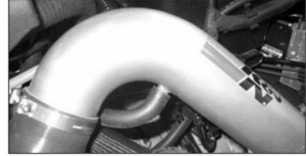
31. Fit the breather hose onto the vent on the K&N Typhoon intake tube as shown. Re-install the battery air breather tube which was removed in step 6 to the vehicle.
