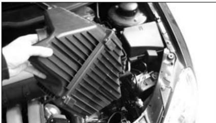
4. Carefully remove the complete air box assembly from the vehicle.
