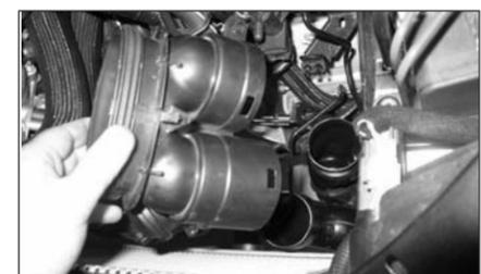
15. Remove the vacuum hose from the top of the air intake assembly and remove the complete air intake assembly from the vehicle.
