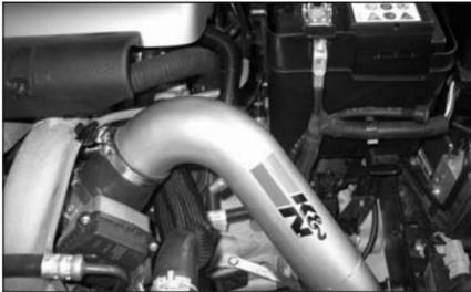
25. Fit the K&N Typhoon intake tube into the silicone hose using the #300 barrel clamp supplied. (Do not fully tighten yet!) **NOTE:** always clean the inside of the tube first.
