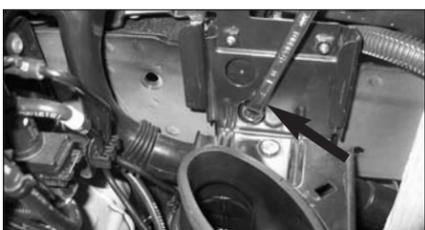
5. Undo the indicated bolt, then, remove the airbox mounting bracket from the vehicle.
