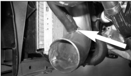
27. Fit the air pump hose onto the vent on the K&N Typhoon intake tube as shown.
