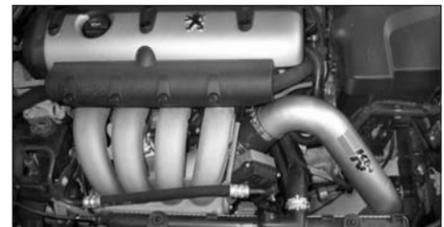
33. Reconnect the negative battery terminal and double check that everything is tight and properly positioned before starting the vehicle.
