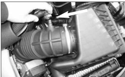
2. Remove the breather hose from the intake tube as shown. Release the 2 hose clamps and remove the intake tube from between the air box and the throttle body.
