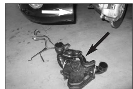
16. Carefully remove the complete resonator box assembly from underneath the vehicle by pulling it backwards.
