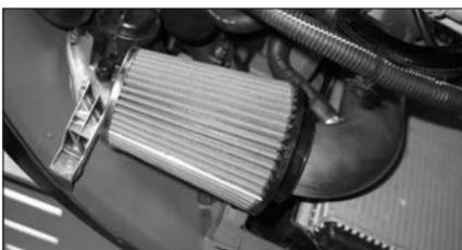
28. Fit the filter onto the K&N Typhoon intake tube using the #44 hose clamp supplied.
