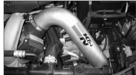
32. Align the intake tube for best fit and clearance, then, firmly tighten the hose clamp and M6 nut. To provide more clearance between the filter and the arch liner you can insert the tube further into the silicone hose.
