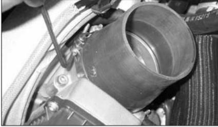
24. Fit the silicone stepped hose onto the throttle body using the #350 barrel clamp supplied. To tighten the barrel clamp, use the small 9/64" Allen wrench provided.
