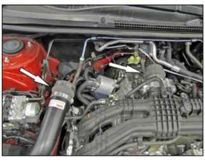
17. Install the provided hump coupler hoses onto the throttle body and the K&N<sup>®</sup> intake tube as shown and secure with the provided hose clamps.
