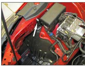
15. Remove the bolt that secures the electrical junction block to the inner fender.
