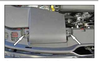
5. Remove the two retaining clips and then remove the fresh air duct from the vehicle.
