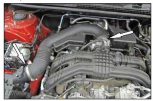
4. Loosen the two hose clamps that secure the intake tube to the throttle body and air filter housing. Remove the intake tube from the vehicle.
