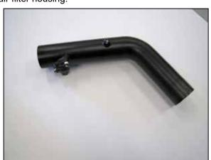
11. Install the mass air sensor into the  $K\&N^{\circledcirc}$  intake tube and secure with the hardware provided.
