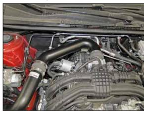
19. Install the K&N® intake tube into the hump couplers, adjust both tubes for best fit and then secure the hose clamps and the tube mount to the heat shield.
