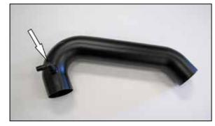
18. Install the provided 90° vent fitting into the K&N® intake tube as shown.
