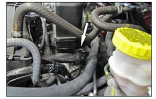
3. Disconnect the crank case vent line from the intake plenum.
