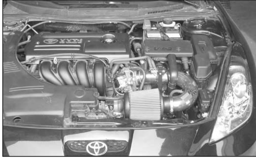
46. Re-connect the negative battery cable and double check that everything is tight and properly positioned before starting the vehicle.
