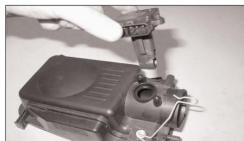
14. Remove the screws from the MAS, then, remove the MAS from the air box as shown.
