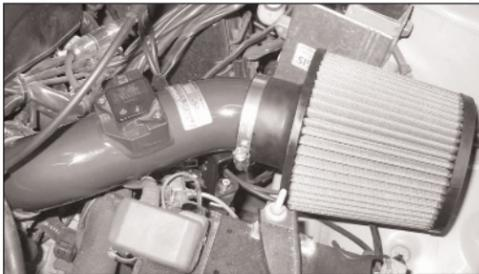
22. Install the Air Filter onto the Typhoon tube and secure with the provided hose clamp as shown.
