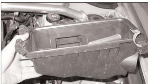
9. Remove the air box base from the vehicle as shown.
