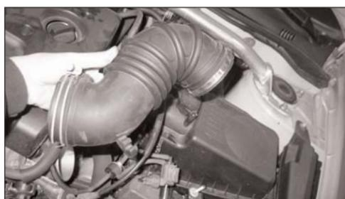
4. Remove the intake tube from the throttle body and the air box. The hose clamps are being used later on.
