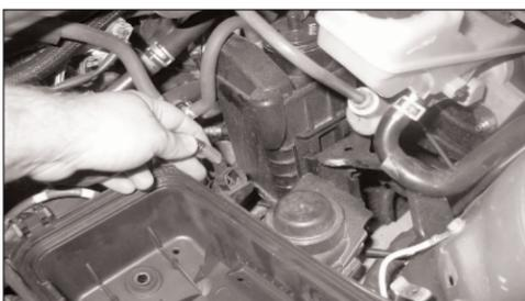
8. Unclip the wire harness from the air box base as shown.
