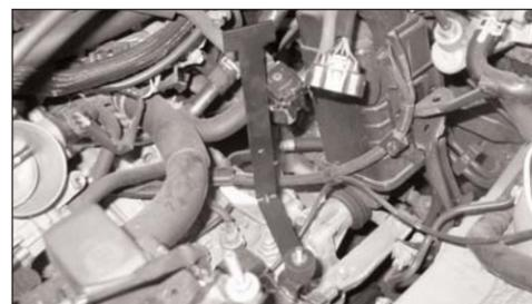
12. Fit the "L" bracket to the original air box mount using the rubber mounted stud as shown.
