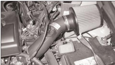
23. Adjust the filter assembly for clearance, then, firmly tighten all hose clamps and hardware connections!
