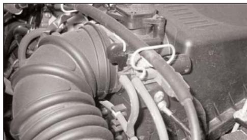
3. Remove the throttle cable from the air box as shown.
