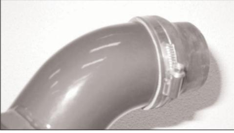
18. Fit the stepped silicone sleeve on the tube using the original hose clamp removed earlier.
