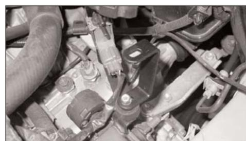
13. Fit the "C" bracket to the rubber mounted stud using a waved washer and nylock nut supplied, but do not tighten completely.
