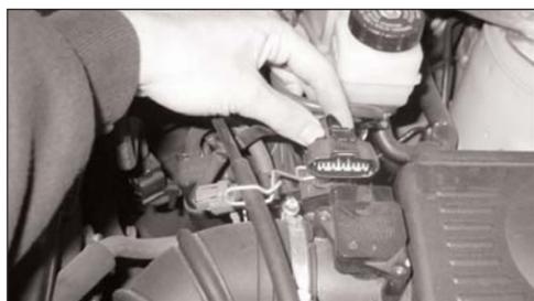
2. Disconnect the mass air sensor (MAS) electrical connection as shown.
