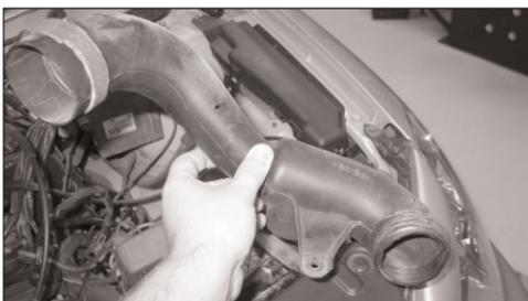
11. Remove the air inlet duct from the vehicle as shown.
