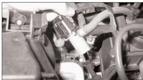
5. Remove the PWM vacuum switching valve from the air box lid.
