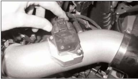
24. Re-connect the MAS electrical connection as shown.
