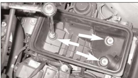
7. Loosen and remove the three bolts that secure the air box base to the vehicle as shown.
