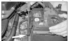
17. Depress the two lower release tabs on each side of the secondary battery cover as shown.
