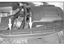
49. Reinstall the inner core support cover as shown.
