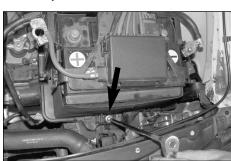
14. Remove the battery hold down block as shown.
