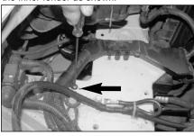
26. Using the provided plastic clamp secure the harness to the inner fender using the provided hardware as shown.
