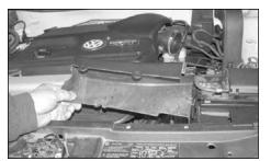
12. Remove the inner core support cover, which is secured by two screws.
