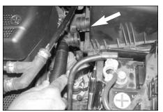
7. Disconnect the air pump vent hose as shown.
