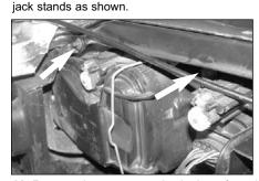
22. Remove the two upper plastic rivets from the inner plastic headlight cover as shown.
