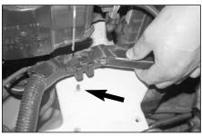
25. Remove the wire harness from the stud on the inner fender as shown.
