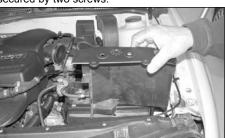
13. Remove the outer core support cover, which is secured by two screws.
