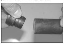
33. Install the provided plastic fitting onto the silicone hose from step 32.
