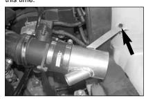
31. Slide the K&N short ram intake tube into the silicone hose and secure the tube bracket to the original air cleaner mounting hole using one of the air cleaner bolts removed earlier.
