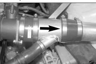
38. Slide the hose over the short ram tube, adjust for best fit and clearance and tighten all hose clamps and hardware as shown.
