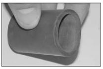
32. Cut a 2-1/2" length of hose from the provided silicone hose as shown.
