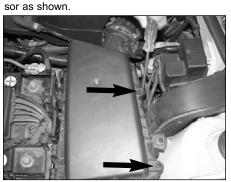
$\ensuremath{\text{6.}}$  Remove the air cleaner cover screws as shown.
