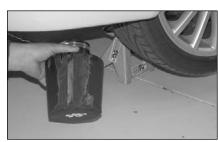
40. From underneath the vehicle install the Filter onto the cold air tube and secure with the provided hose clamp.
