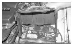
18. Remove the battery cover as shown.
