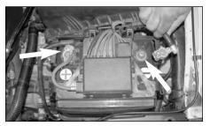
3. First disconnect the negative battery cable, then disconnect the positive battery cable as shown.
