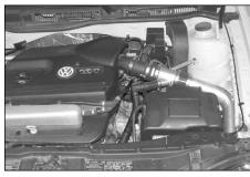
51. This K&N Typhoon intake kit has been designed to be used in two different configurations. In the case of inclement weather, the cold air tube can be removed and the filter can be clamped onto short ram tube located in the engine compartment to avoid the possibility of ingesting water into the engine.
