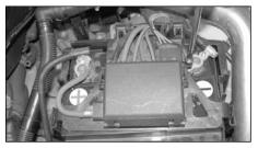
45. First reconnect the positive then the negative battery cable as shown.
