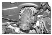
28. Reinstall the mass air sensor into the stock rubber intake hose as shown, but do not tighten at this time.
