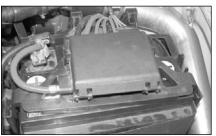
43. Reverse the removal process and slide the battery fuse/harness onto the battery cover as shown
