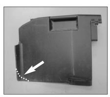
47. Trim the corner of the outer core support cover to provide clearance for the cold air tube as shown.
