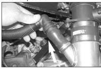
35. Reconnect the hard line to the plastic fitting as shown.
