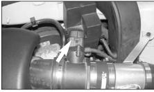
50. Reconnect the mass air sensor electrical connection as shown.
