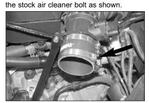
30. Install the silicone hose and hose clamps onto the mass air sensor but do not tighten at this time.
