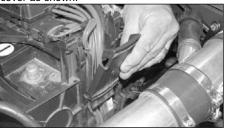
44. Slide the rear battery harness cover back onto the battery cover as shown.
