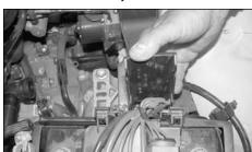
15. Slide the rear battery harness cover upwards and remove from the battery cover as shown.
