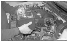
19. Remove the battery as shown.
