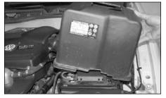
2. Depress the tabs on the side of the battery cover and remove as shown.
