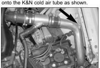
37. Slide the cold air tube into the hole in the inner fender, then, line up the bracket with the stud on the inner fender and secure with the provided hardware as shown.
