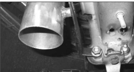
20. Mount the "L" bracket onto the thread of the front beam using the M10 washer and M10 nut supplied. Do not fully tighten at this moment.
