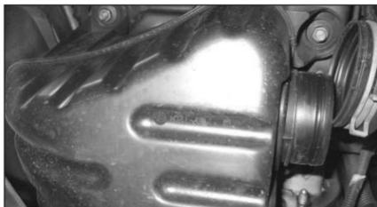
11. Remove the three bolts securing the resonator box to the vehicle.
