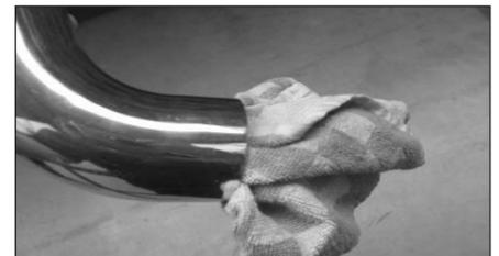
16. Clean the inside of the new intake tube with water and a towel.
