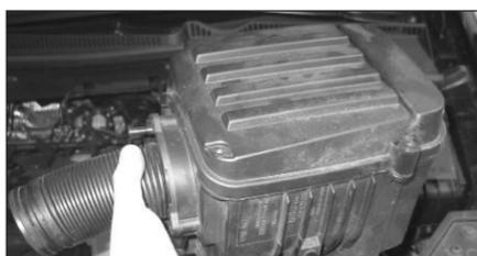
6. Remove the complete air box from the vehicle by pulling the air box upwards.
