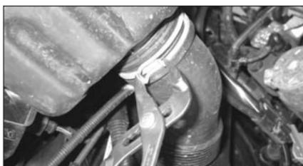
10. Unclip the intake snorkel hose from the resonator box using the pliers as shown.
