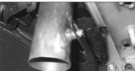
21. Fit the new intake tube onto the "L" bracket using the M6 washer, M6 waved washer and M6 bolt supplied. Do not fully tighten at this moment.
