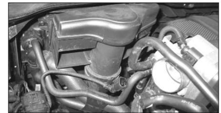
14. Unclip the intake snorkel hose from the intake snorkel as shown.
