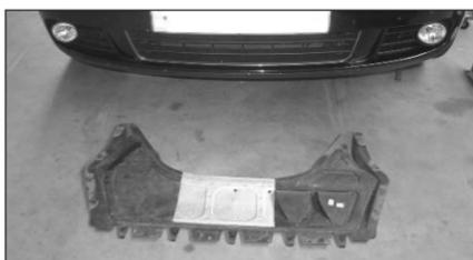
9. From underneath the car remove the under-tray as shown.
