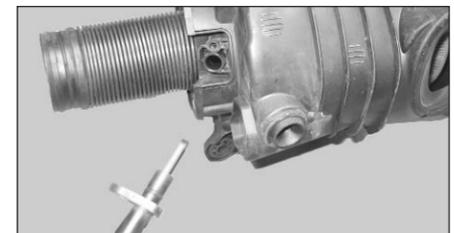
15. Remove the temperature sensor from the air box as shown.
