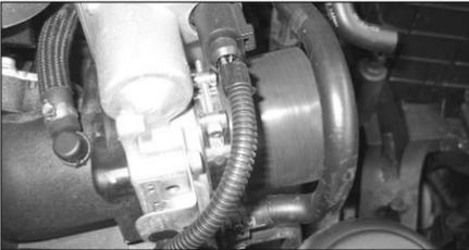
18. Fit the silicone sleeve onto the throttle body using the #40 hose clamp supplied.
