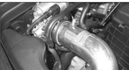
19. Fit the new intake tube into the silicone sleeve using the #44 hose clamp supplied. Do not fully tighten at this moment.
