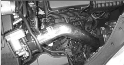
24. Align the new intake tube for best fit and clearance, then, firmly tighten the hose clamp and M6 and M10 nut.
