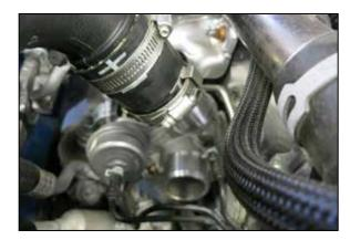
7. Loosen the hose clamps that secure the hot side charge tube to the turbo and intercooler and then remove the charge tube from the vehicle.
