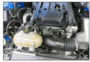
18. Reinstall the complete intake system and reconnect the factory BOV hose to the intake tube.
