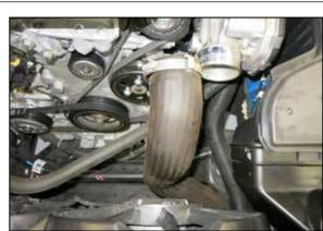
5. Loosen the hose clamps that secure cold side charge hose to the throttle body and inter cooler and then remove the cold side charge hose from the vehicle.
