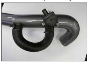
9. Install the BOV onto the K&N hot side charge tube and secure with the factory hardware removed in the previous step. Install the factory BOV hose onto the K&N hot side charge tube.
