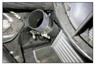
15. Install the provided step coupler onto the cold side of the inter cooler with the provide clamps, do not tighten.
