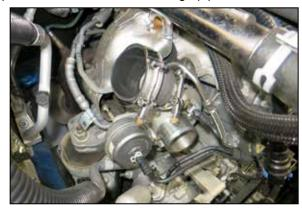
11. Install the provided step coupler into the turbo outlet with the provided clamps, do not tighten the clamps.
