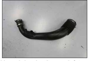
4. Loosen the hose clamp the secures the factory intake tube to the turbo inlet and then remove the intake tube from the vehicle.
