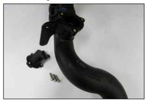
8. Remove the three bolts that secure the BOV to the factory charge tube and remove the valve from the tube. Release the spring clamp and disconnect the BOV hose from factory hot side charge tube
