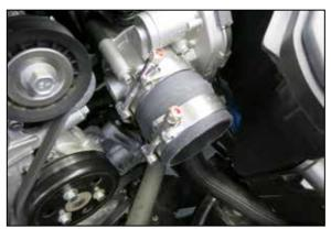
14. Install the provided hump coupler onto the throttle body with the provided clamps, do not tighten the clamps.
