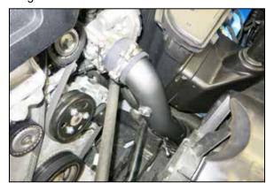
16. Install the K&N cold side charge tube into the couplers, align for best fit and then tighten the clamps.
