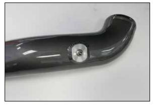
10. Apply thread sealant to the provided 1/8npt plug and then install the plug into the accessory port of the K&N cold side charge pipe.
