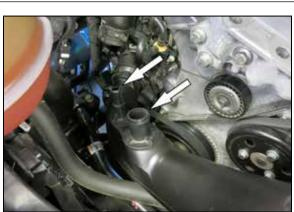
3. Release the spring clamp that secures the BOV hose to the intake tube and then disconnect the CCV line quick disconnect fitting from the intake tube.
