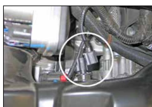
4. Disconnect the inlet air temperature air sensor electrical connection.
