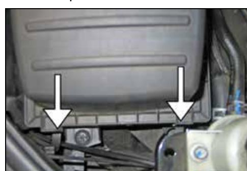
6. Release the two upper air box retaining clips.
