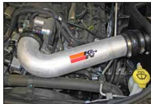
21. Install the K&N® intake tube into the silicone hump hose and then into the silicone hose at the throttle body, secure the intake tube with the provided hose clamp.
