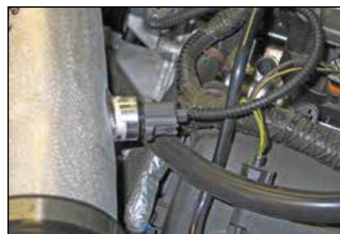
23. Connect the inlet air temperature sensor extension harness into the factory electrical connection and then connect the other end into the inlet air temperature sensor as shown.
