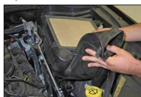
9. Lift up the lower air box to dislodge it from the mounting grommets and then remove the lower air box from the vehicle. Some vehicles may have a power steering line attached to the airbox that will need to be unhooked.
