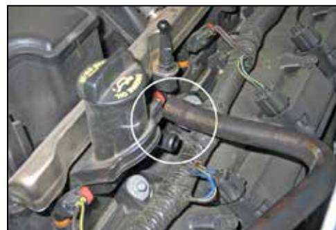
5. Disconnect the crank case vent hose from the valve cover port.
