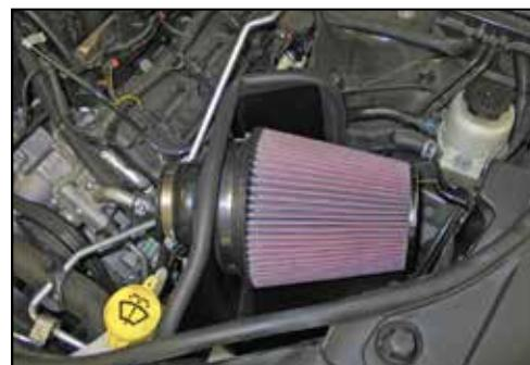
16. Install the K&N® air filter onto the adapter and secure with the provided hose clamp.
