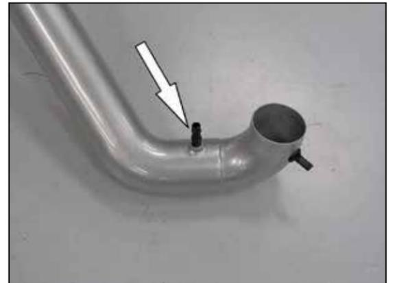
21. Install the provided vent fitting into the K&N® intake tube as shown. **NOTE: Plastic NPT fittings are easy to cross thread. Install the vent fitting "hand" tight, then turn it two complete turns with a wrench.**
