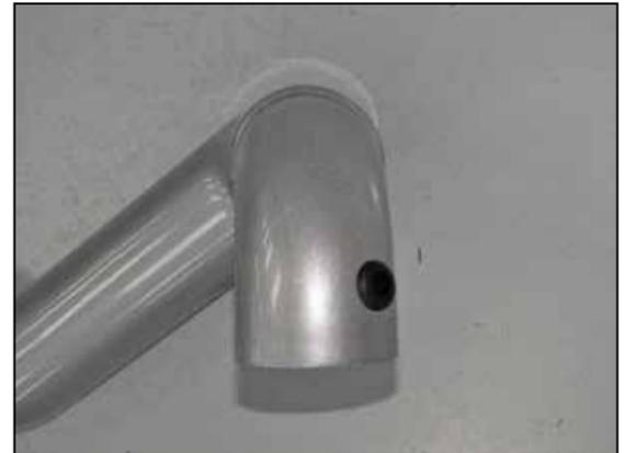
18. Install the provided grommet into the K&N® intake tube.
