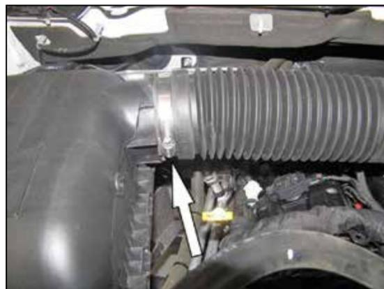
4. Loosen the hose clamp securing the intake hose to the factory air box.
