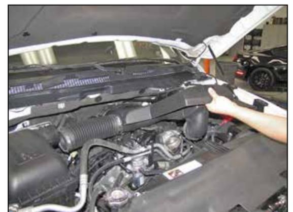
5. Lift up the intake plenum to dislodge it from the mounting grommets and then remove the plenum from the vehicle.
