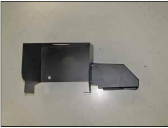
7. Install the K&N® fresh air intake scoop onto the K&N® heat shield and secure with the provided hardware.
