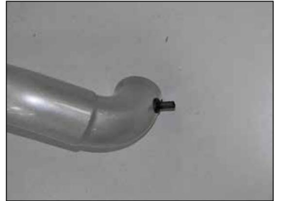
20. Install the inlet air temperature sensor into the grommet installed into the K&N® intake tube. **NOTE: Remove the factory sealing O-ring from the sensor before installation.**
