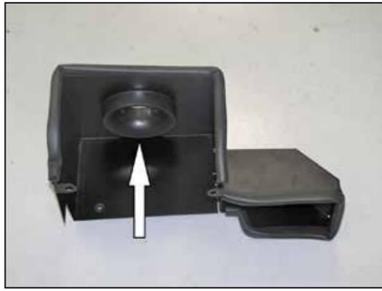
12. Install the K&N® air filter adapter into the heat shield and secure with the provided hardware.
