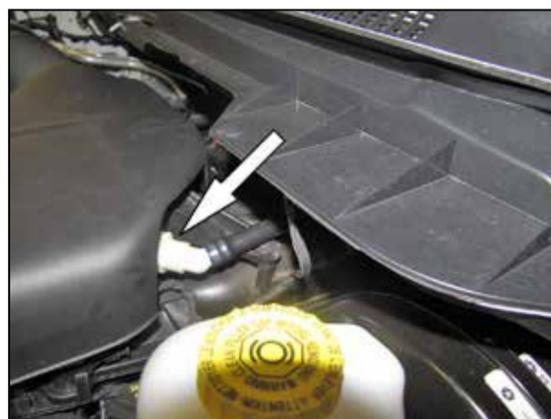
3. Disconnect the crank case vent from the intake plenum.
