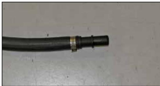
24. Install the provided quick disconnect fitting into the provided crank case vent hose and secure with the provided hose clamp.
