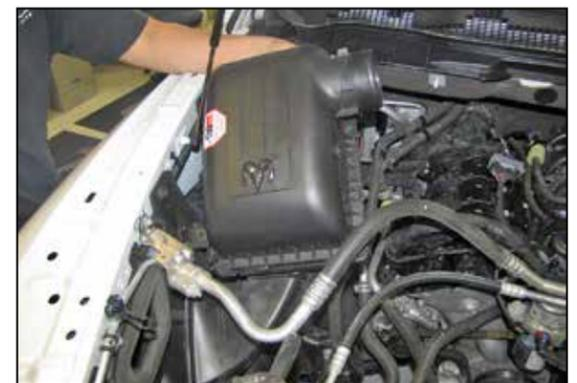
6. Lift the air box assembly off of the mounting studs and then remove the air box from the vehicle. **NOTE: K&N Engineering, Inc., recommends that customers do not discard factory air intake.**
