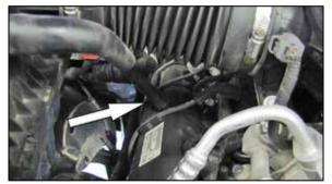
3. Disconnect the crank case vent hose from the valve cover fitting and then lift up and remove the air filter housing and intake tube to remove it from the vehicle.
