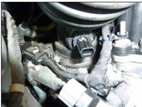
9. Loosen the hose clamp that secures the intake tube to the throttle body and then remove the intake tube from the vehicle.
