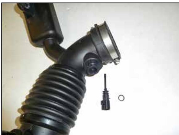
10. Remove the IAT sensor from the factory intake tube and remove the O-Ring from the sensor.
