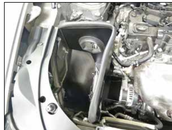
17. Install the heat shield into the vehicle as shown so the mounting studs insert into the grommets.
