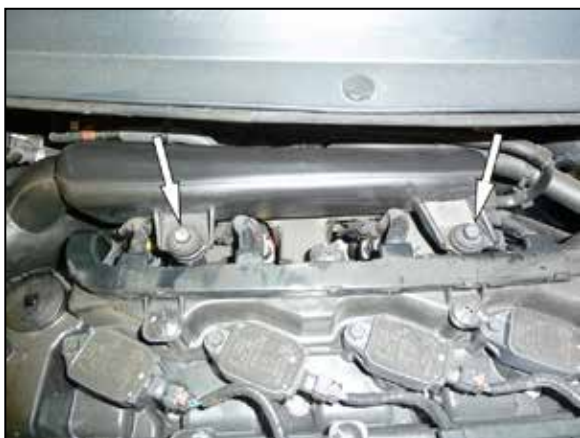
8. Remove the two bolts shown that secure the factory intake tube.
