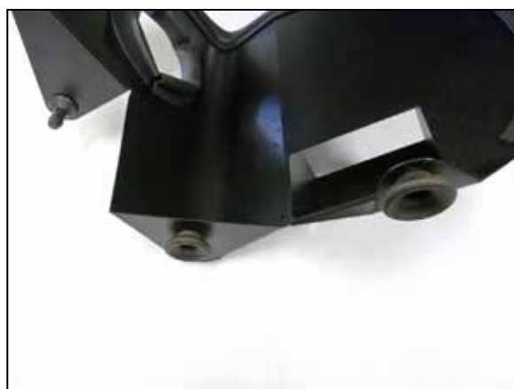
16. Install the two factory air filter housing mounting brackets onto the heat shield as shown.
