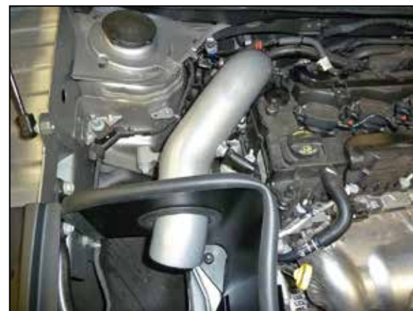
19. Install the K&N intake tube into the heat shield and then into the coupler, adjust the tube for best fit and then secure with the provided hose clamp.
