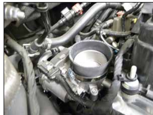
18. Install the provided coupler onto the throttle body and secure with the provided hose clamp.
