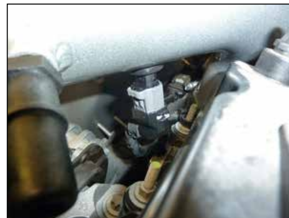
20. Reconnect the IAT sensor electrical connection.
