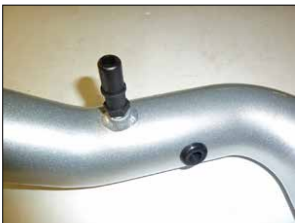
11. Install the provided grommet and quick disconnect fitting into the K&N intake tube as shown.
