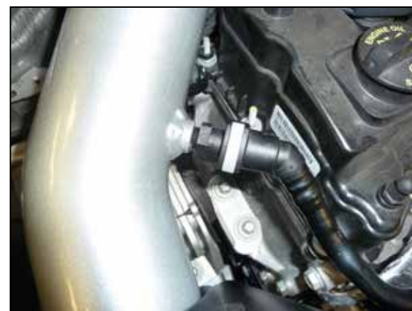
21. Reconnect the PCV to the Quick connect fitting installed into the K&N intake tube.
