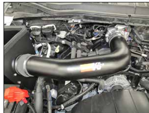
19. Install the K&N® intake tube into the hump coupler and then into the step coupler at the throttle body, adjust the tube for best fit and then secure with the provided hose clamps.
