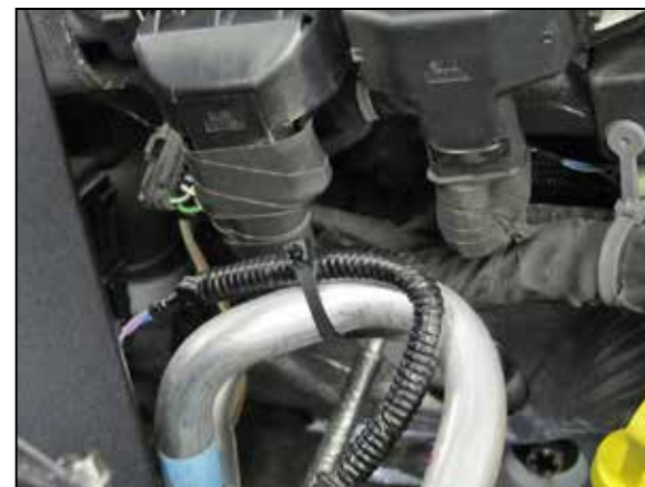
17. Secure the wiring pigtail from step #5 to the A/C line with the provided tie wrap.
