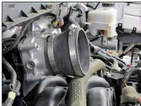
16. Install the provided step coupler (08497) onto the throttle body and secure with the provided hose clamp.
