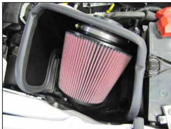
14. Install the heat shield assembly into the vehicle so that the mounting studs insert into the factory air filter housing grommet locations.
