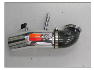
18. Install the provided angled coupling hose (084087) onto the intake tube as shown. NOTE: Do not secure the hose at this time as it will need to be adjusted.
