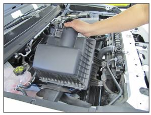
8. Remove the air filter housing assembly from the vehicle.
