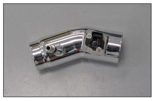
16. Install the mass air sensor into the K&N® adapter and then install the assembly into the K&N<sup>®</sup> intake tube and secure with the provided hardware.
