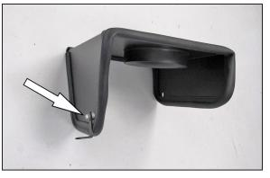
12. Install the heat shield mounting bracket (070812) onto the heat shield using the provided hardware and spacer.
