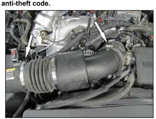
2. Loosen the two hose clamps that secure the intake tube to the air filter housing and intake plenum, then remove the intake tube from the vehicle.
