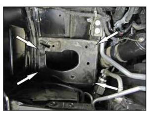
5. Remove the four bolts that secure the air filter housing mounting plate to the inner fender and then remove the mounting plate from the vehicle. NOTE: Three of the factory bolts will be reused in a later step.
