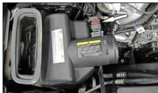
4. Release the red locking tab and then disconnect the mass air sensor electrical connection. Unhook the coolant bypass hose from the air filter housing. Lift the air filter housing up to dislodge it from the mounting grommets and remove it from the vehicle. **NOTE: K&N Engineering, Inc., recommends that customers do not discard factory air intake.**
