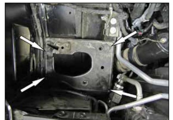
5. Remove the four bolts that secure the air filter housing mounting plate to the inner fender and then remove the mounting plate from the vehicle. **NOTE: Three of the factory bolts will be reused in a later step.**
