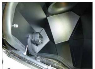
14. Install the heat shield assembly into the vehicle
