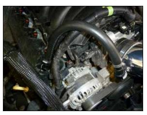
24. Connect the crank case vent hose assembly to the valve cover port and then to the fitting installed into the intake tube.
