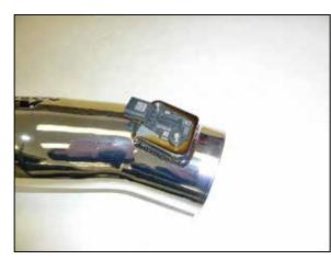
21. Remove the mass air sensor from the factory housing. Install the mass air sensor into the K&N<sup>®</sup> intake tube and secure with the provided hardware.
