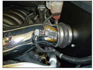
25. Connect the mass air sensor electrical connection.
