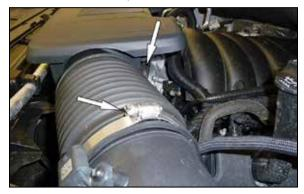
4. Loosen the hose clamps that secures the intake plenum to the air filter housing and to the throttle body. Disconnect the plenum connections at the air filter housing and then rotate the plenum counter clockwise to disengage the keyed mount and separate it from the throttle body. NOTE: The wiring harness anchored to the intake plenum will need to be detached before removing the plenum from the vehicle.
