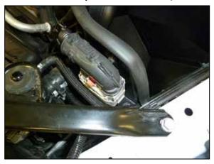
15. Connect the wiring bulk connector onto the bracket installed onto the heat shield.
