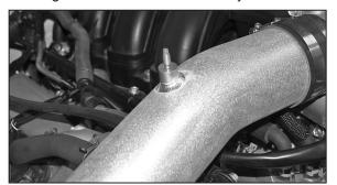
30. Install the engine cover mounting stud into the threaded stand off on the K&N $^{\odot}$  intake tube as shown.
