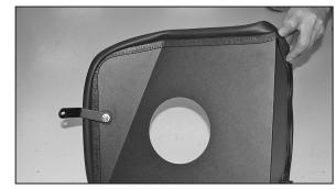
13. Secure the mounting bracket to the rubber mounted studs to the original air box mounting holes as shown.
