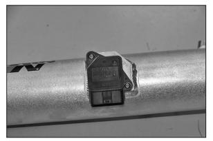
19. Install the mass air sensor into the K&N<sup>®</sup> intake tube with the hardware provided.
