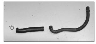
22. Remove the crank case vent hose from the valve cover and then remove the factory clamp and outer cover from the crank case vent hose as shown.
