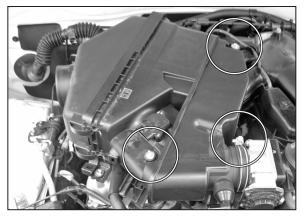
9. Loosen the hose clamp at throttle body, then remove the two bolts that secure air box to engine.
