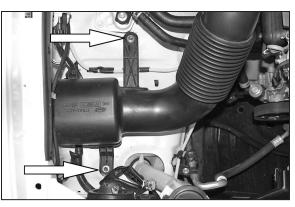
4. Remove the two bolts which secure the intake resonator to the fender well.
