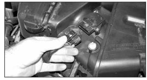
6. Disconnect the two mass air wire harnesses retaining clips from air box, then disconnect the mass air sensor electrical connection.
