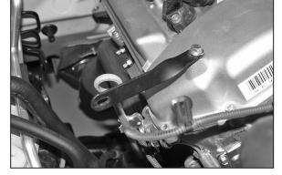
20. Install the tube mounting bracket onto the threaded boss on the valve cover with the provided hardware as shown. **NOTE: Do not tighten completely at this time.**  25. Remove the stock vacuum hose from the fuel pressure regulator, then install the provided silicone hose to the fuel pressure regulator and then onto the K&N<sup>®</sup> intake tube as shown.
