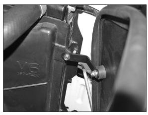
16. Secure the mounting bracket to the fan shroud with the original bolt.
