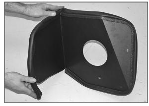
11. Apply the edge trim to the K&N<sup>®</sup> heat shield as shown above, trim if needed.
