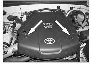
32. Install the engine cover and secure with the factory mounting nuts removed in step #2.
