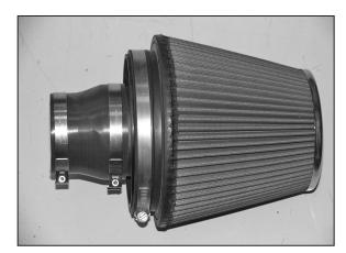
27. Install the silicone hose (084055) onto the Air Filter assembly as shown and secure with the provided hose clamp.
