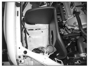
15. Install the heat shield into the vehicle so that the mounting tabs rest on the rubber mounted studs installed in step #14.
