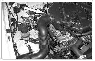
3. Loosen the intake tube hose clamp at the air filter assembly.
