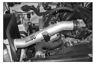
21. Install the K&N<sup>®</sup> intake tube into the silicone hose at the throttle body and align the mounting stand off with the bracket installed in step #20. Secure the intake tube with the hose clamp and hardware provided.
