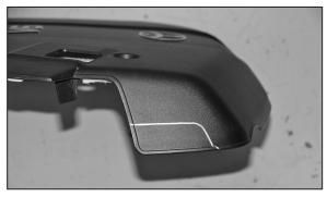
31. Using the provided template, mark the trim lines onto the engine cover and then cut with the appropriate tool.
