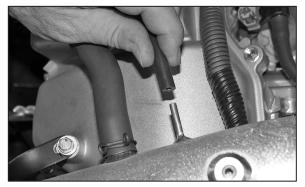
14. Install the two remaining rubber mounted studs to the original air box mounting holes as shown.
