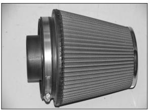
26. Install the filter adapter into the Air Filter as shown.
