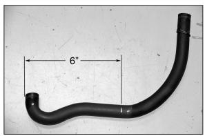
23. Measure 6" from the end of the crank case vent hose as shown and cut the hose.
