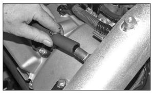
24. Reinstall the crank case vent hose into the valve cover and then connect the cut end to the  $K\&N^{\mbox{\sc sn}}$  intake tube as shown. Secure the vent hose with the factory spring clamps.
