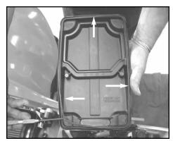
22. Remove the o-ring from the groove on the stock air box lid. Reinstall the o-ring in the X-STREAM<sup>™</sup>  $POWERLID^{TM}$  groove.
