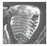
30. Install the front plate on the K&N® air filter. NOTE: Make sure the front plate is completely seated onto the K&N® air filter.
