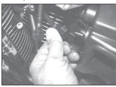
8. Unplug the wiring from the air temperature sensor on the back of the air cleaner assembly.
