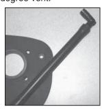
23. Install the second 90 degree vent into the other end of the hose.
