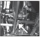
26. Reinstall the breather tube removed in step 6 into the straight vent.
