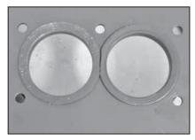
13. Make sure the velocity stacks are completely seated on the back plate.
