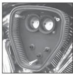
29. Install the K&N<sup>®</sup> air filter onto the backplate. NOTE: Make sure the air filter is completely seated onto the back plate.
