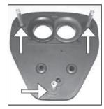
20. Install the buttonhead bolts through the back of the back plate and thread into the spacers. Tighten completely at this time.
