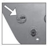
18. Install the air temperature sensor into the top left grommet.
