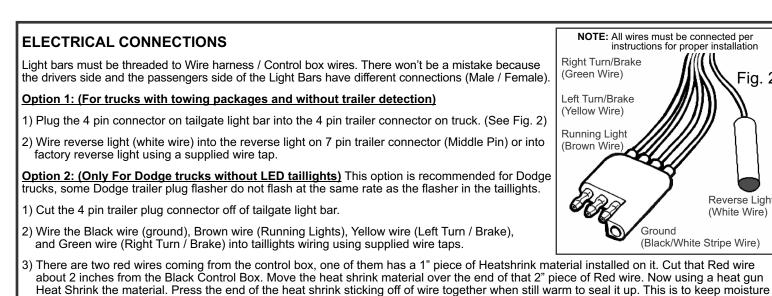
out of the wire. 4) Now Pull the other Red wire from the black PVC tubing (enough to reach the +12V power on the 7 pin connector) and wire to the +12V power on the 7 pin trailer connector using a supplied wire tap. Some trucks do not provide a constant +12V unless a trailer is plugged into the 7 pin trailer connector. If this is the case, a separate 16GA or bigger wire may need to be ran from the positive on the battery, additional
