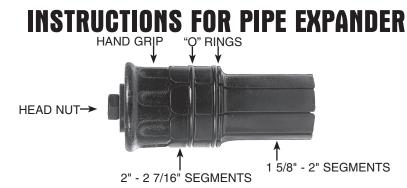
Holding tool by handgrip, insert it into pipe. If pipe is less than 2" diameter, the small end is used. On pipes 2" and over, push right on in until the large segments will contact. Expand by turning head nut with a wrench. Tool will expand smoothly and easily and will round up pipe end quickly. The tool does not turn in the pipe.
