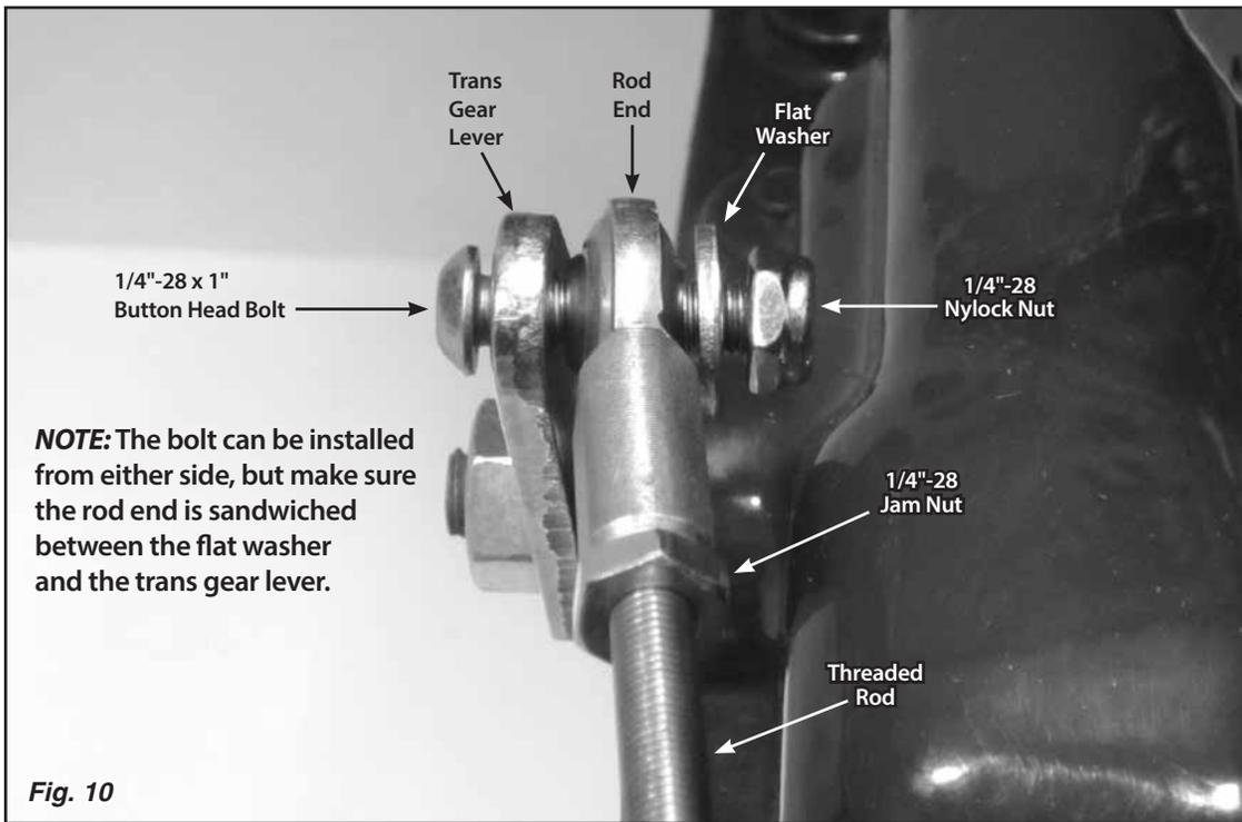
**NOTE:** The bolt can be installed from either side, but make sure the rod end is sandwiched between the flat washer and the trans gear lever.
