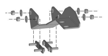
Insert (2) 10mm Double Bolt Plates up into the open end of driver/left side frame channel and out through the Frame Bracket.
