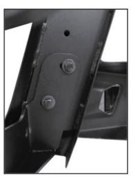
Attach each mounting bracket to the bull bar with (2) bolt assemblies
