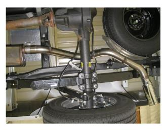
**Step 3.** Finish by installing the Tail Pipe Assembly to the Tail Pipe Extension using the supplied 3.00" clamp, fitting the welded hanger into rubber insulator.
