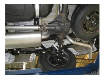
**Step 1.** To remove the OEM exhaust system, you will to need to cut the pipe beind the muffler before it goes over the axle. You can then disengage the welded hangers from the OEM rubber insulators and remove the tailpipe. Unbole the flange attaching the OEM Resonator to the catalytic converter. Do not damage or discard the OEM fasteners or rubber insulators, as they will be reused to mount the new system. Disengage the muffler hangers and remove the OEM exhaust from the vehicle.
