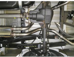
**Step 2.** Begin by fastening the Resonator Assembly to
