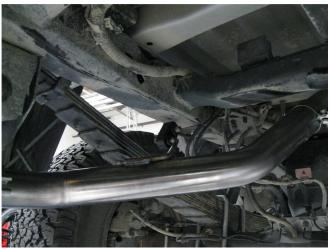
**Step 3.** Next you will need to use the supplied U-Clip nut and attach them to the recieving cut outs in the bottom of the frame member. Fasten the supplied hanger assemblies to the frame members using the supplied bolts on both the Driver and Passenger side. Then install the Tail Pipe Assemblies to the Tail Pipe Extensions using the supplied 2.50" clamp, fitting the welded hangers into rubber insulators.
