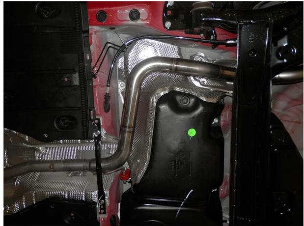
**Step 2.** Begin installation of the new system by attaching the Inlet Pipe to the factory outlet using the OEM clamp and fit the hangers into the rubber insulators. Leave all clamps loose until final adjustment.
