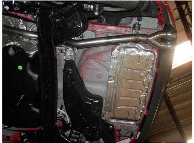
**Step 3.** Next Install the Tailpipe Assembly using the supplied 2.50" clamp and fit the welded hanger into the rubber insulator.
