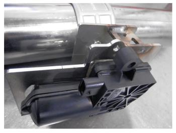
**Step 4.** Before installing your new exhaust system attach the OEM valve motors to each valve using the supplied hardware. The alignment spring on the motor will need to be engaged into the keyway slot of the new valve.
