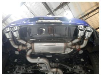
**Step 6.** Loosely install Muffler Assembly using the supplied clamp. Attach the welded hangers to the rubber insulators. Re-attach both electrical connectors to the exhaust valve motors.
