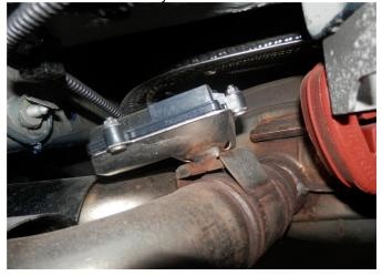
**Step 3.** Once the OEM exhaust system has been removed undo the three nuts attaching each exhaust valve motor to the valve and remove.
