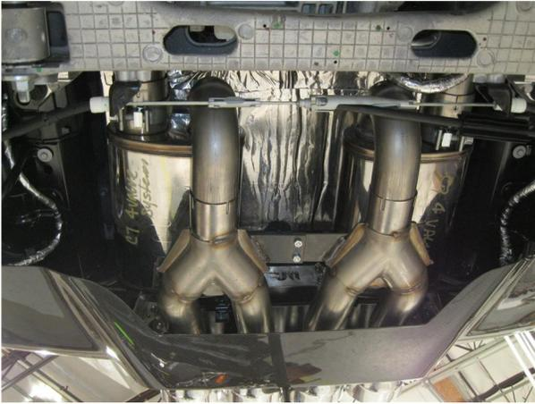
**Step 4.** Once the rear valance is back in place, loosely fasten the Tip sub-assemblies together while on the ground using the supplied fasteners. Now you can attached the Tip assembly to the Muffler assemblies using the provided 2.50" clamps. Plug the wiring into the valve motors checking for clearance.
