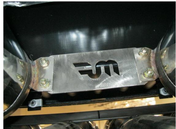
**Step 3.** Next, Loosely attach the Muffler Assemblies to the Inlet pipes using the provided 3.00" clamps. You will then need to fasten the provided cross bracket in place between the two muffler assemblies using the provided 1/4" fasteners. Insert all hangers into the rubber isolators. At this point you can re-install the rear valance.
