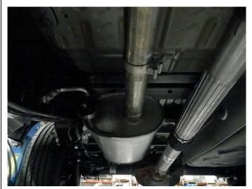
**Step 1.** To remove the OEM exhaust system, loosen the clamp attaching the system inlet pipe to the resonator outlet pipe. Disengage all welded hangers from the OEM rubber insulators. Do not discard the OEM clamp or damage the rubber insulators as they will be needed to mount your new MAGNAFLOW system.
