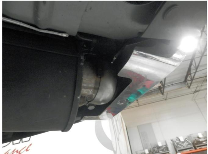
**Step 8.** To retain the OEM tips on your vehicle select the two OEM Tip Assemblies. The drivers side will be slightly longer. Loosely attach each pipe inlet to the Over Axle Pipes outlets using the OEM clamps. Engage the welded hangers for each to the rubber insulators.
