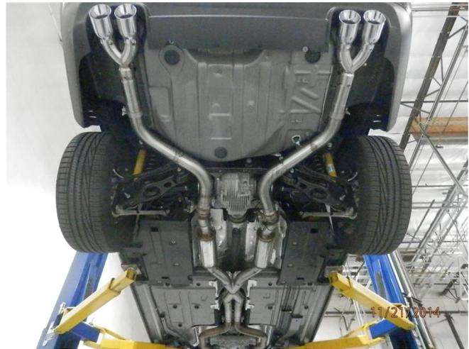
**Step 9.** To install the Quad Tip option supplied you will first need to remove the OEM tips from the vehicles valence. Remove the four bolts attaching each tip. Once the tips are removed install the Quad Tip Tailpipe Assemblies using the supplied 3.00" clamps. Locate both welded hangers to the rubber insulators.
