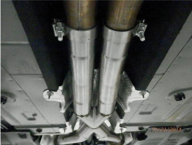
**Step 6.** Begin installation of the new system by slipping the inlet pipes of the X-Pipe Muffler Assembly over the catalytic converter outlets. Loosely secure using two of the supplied 2.75" clamps. Orientation of the Muffler Assembly can be confirmed by the MF logo being "upright" after installation.
