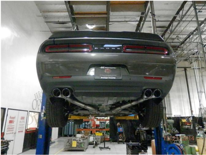
**Step 10.** Once a final position has been chosen for the new exhaust system, evenly tighten all clamps from front to rear using the torque specifications on page one of the instructions. Inspect all fasteners after 25-50 miles of operation and re-tighten if necessary.
