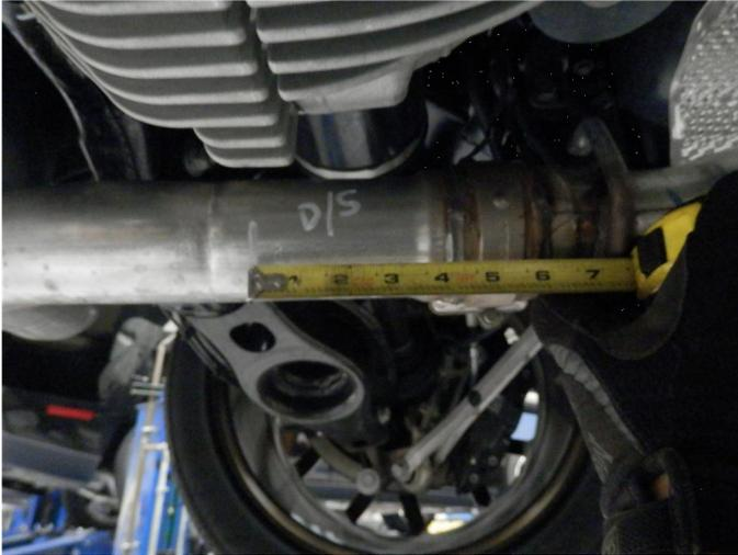
**Step 1.** Begin removal of the OEM system by cutting both sides of the systems exhaust pipes. Four cuts will need to be made. For the drivers side cut 4" rearward of outlet weld on the exhaust control valve as shown in the attached picture.
