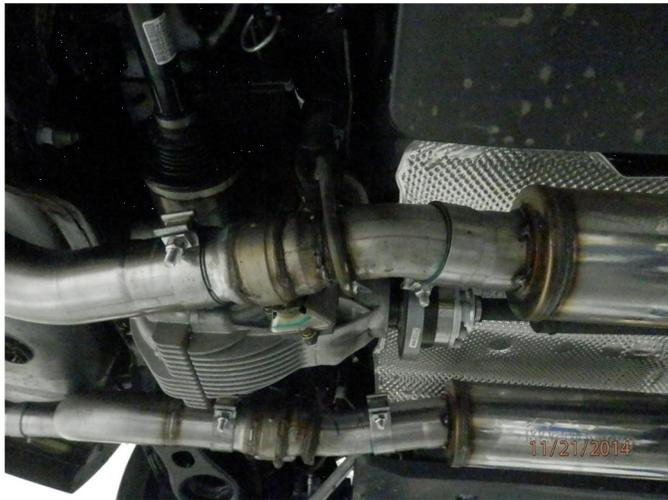
**Step 7.** Next, loosely fasten the X-Pipe Muffler Assembly outlet pipes to the OEM control valve outlet that you have just cut using the supplied 2.75" clamps. Attach the two Inlet Pipes in a similar fashion to the outlet of the control valve. At this point you have two options for tips. Magnaflow supplies a quad tip setup or an extension pipe assembly to allow for the original OEM tips. Select the desired option before continuing the installation.
