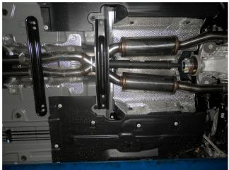
**Step 2.** Begin installation of the new system by attaching the Driver and Passenger side (Passenger is the longer of the two pipes) inlet pipes to the outlets of the OEM system using the supplied 2.50" clamps. Next attach the Resonator Assembly to the inlet pipes with supplied clamps and insert the hangers into the rubber insulators.
