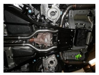
**Step 3.** Next attach the Mid Pipe Assemblies to the X-Pipe using the supplied 3.00" clamps and fitting the hangers into the rubber insulators.
