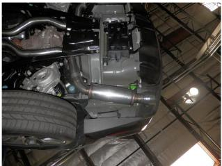
**Step 4.** Finish the initial installation by fitting the Muffler Assemblies onto the Mid pipe Assemblies using the supplied 3.00" clamps and inserting the hangers into the rubber insulators.
