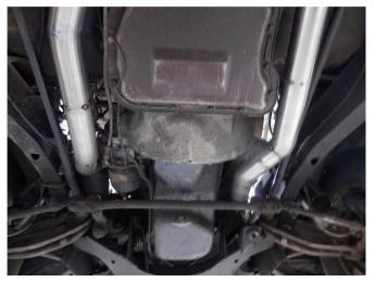
**Step 1.** This install sheet assumes you have already removed the OEM exhaust system. Identify the drivers side and passengers side Manifold Pipes.
