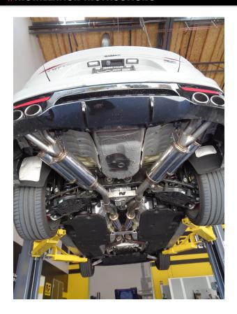
Step 4: Once a final position has been chosen for the new exhaust system, evenly tighten all clamps from front to rear using the torque specifications on page one of these instructions. Tighten fasteteners for Muffler brace and install factory underbody brace. Inspect all fasteners after 25-50 miles for operation and re-tighten if necessary.
