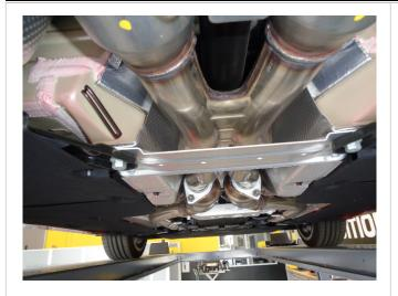
Step 1. To extract the OEM exhaust system you will first need to remove the brace located in front of the factory resonator. Next un-fasten the flanges located behind the catalytic converters and resonator and disengage all welded hangers from the rubber insulators. Do not damage or discard the rubber insulators or fasteners as they will be re-used to mount the new system. You can now remove the exhaust from the vehicle.
