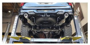
Step 1: To remove the OEM exhaust system unfasten the flange in front of the Y-Pipe and the band clamp behind the "Y". Working front to rear disengage the Tailpipe welded hangers from the rubber insulators and remove the system. (Retain the insulators as they will be needed to mount the new MagnaFlow system.)
