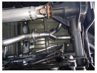
Step 2: Install the new system by attaching the Y-Pipe Assembly to the outlet of the valve mid pipe.
