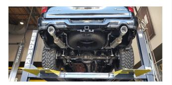
Step 5: Once a final position has been chosen for the new exhaust system, evenly tighten all clamps from front to rear using the torque specifications on page one of the instructions. Inspect all fasteners after 25-50 miles of operation and re-tighten if necessary.
