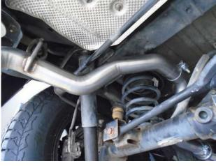
**Step 4.** Install Tail Pipe "A" and Tail Pipe "B" as shown using the supplied clamps and fit the welded hangers into the rubber insulators.
