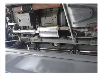
**Step 2.** Being installation of your new system by fitting the Muffler Assembly inlet pipe to the catalytic converter outlet. Locate the welded hanger to the rubber isolator. Secure using the supplied clamp. Be sure to fit the OEM alignment peg in the larger notch. Leave all clamps loose for final adjustment.
