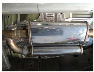
**Step 3.** Attach the Muffler Assembly to the Reasonator Assembly with a supplied 3.00" clamp.
