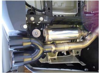
**Step 5.** Complete the installation by attaching both Tailpipe Assemblies to the Y-Pipe Assembly using the Supplied 2.50" clamps.
