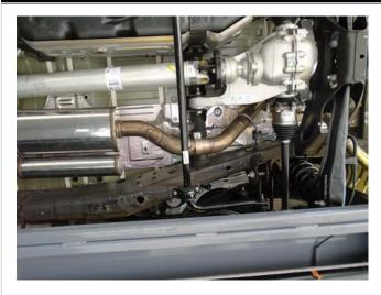
**Step 4.** Next loosely attach the Y-Pipe Assembly to the Muffler Assembly using the supplied clamp. Engage the welded hangers to the rubber insulators.
