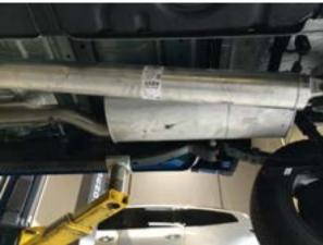
**Step 2:** Working front to rear, with the exhaust system supported, disengage all welded hangers from the rubber insulators and remove. (Retain the rubber insulators as they will be needed to mount the new MagnaFlow system.)
