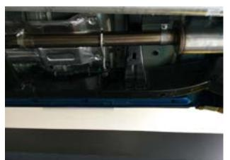
**Step 4:** Next, attach the Oval Muffler to the Extension Pipe using the supplied 3.00" clamp. This exhaust system is configured to allow the user to tune the sound. For a more moderate exhaust sound install the U-pipe Assy and the 4.00" NDT Chamber (as shown) using the suppled 2.50" clamps. For a more aggressive sound see configuration chart below.
