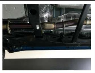
**Step 3:** Begin Installing the new system by attaching the Inlet Pipe assembly to the flanged outlet using the OE hardware.
