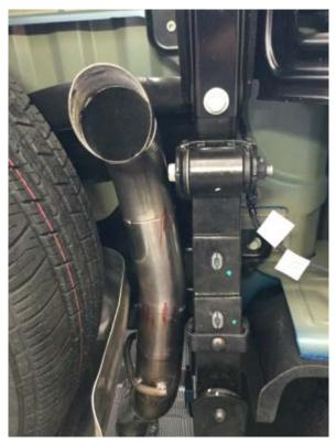
**Step 7:** Installing the Tail Pipe to the Over Axle Pipe outlet using the supplied clamp. Engage the hanger to the OE rubber insulator. Clearances are very tight, make sure there is adequate room after tightening.
