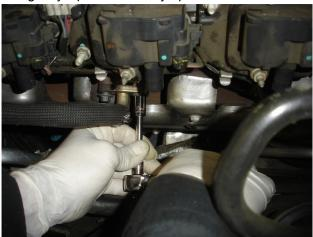
**Step 3.** Unbolt and remove the EGR pipe on the passenger side using a 10mm socket.
