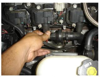
**Step 5.** Disconnect the hose from the EGR pipe on the driver side and remove.
