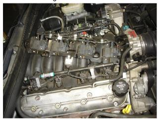
**Step 2.** Remove all spark plug wires from the coils and the plugs, and then set aside. On the passenger side unbolt the coil pack bracket using a 10mm socket and gently flip the assembly up towards the motor.
