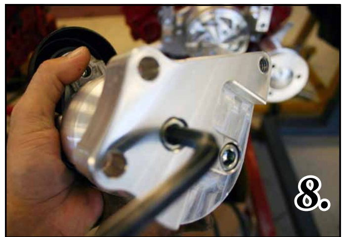
Photo-8 1. Hold Tensioner Body in a vise to remove bolt & washer from tensioner pulley. Note: Bolt is a left handed thread, turn clockwise to remove. Install the Tensioner into the 20256-B Bracket cover use a \frac{3}{8} x 3\frac{1}{4} " SHCS and install the (781-A) cover as shown and bolt into place.
