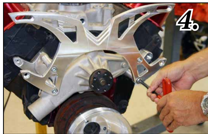
Fig 5. Install \frac{5}{8} "-18 Threaded Alternator Adjustment Bushing (S452) into Rear Alternator Support Bracket as shown.
