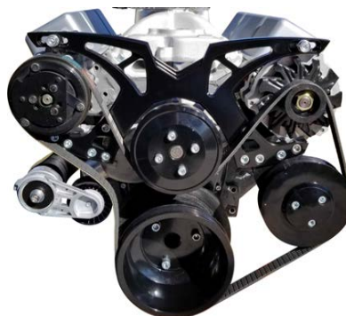
Kits with Type 2 p/s use a 62" 6 rib belt (Dayco 5060620)
