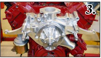
**Photo-4** Install the Main Front Plate (40731-A) to the four studs using four  $\frac{3}{8}$ -16 x  $\frac{3}{4}$ " SHCS (S244).
