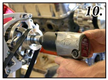
**Photo-11** Push both the Alternator and Power Steering units inwards at the top mounts and install the Install the  $67^{1}/2^{11}$  Inch belt as shown. Slip the supplied March Adjustment Tool (30436) over the two (MM100) bushings at the Alternator an Power Steering sides. Use a wrench to turn the adjustment tool outward to tighten the serpentine belt to 100 ft. lbs.
