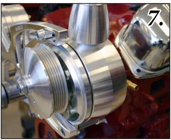
**Photo-8** Install the two Idlers (740-A) to the main plate using two (S666)  $\frac{3}{8}$ " washers and two  $\frac{3}{8}$  x  $1\frac{3}{4}$ " Hex Bolts (S321). Install the Idler Covers (302-A) with three  $\frac{8}{32}$  x  $\frac{3}{8}$ " SHCS (S022).
