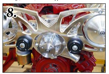
**Photo-9** For O.E.M. Balancers Install the Crank pulley (10366-A) using (6)  $\frac{5}{16}$  x  $\frac{7}{8}$ " SHCS (S144) and using the (10367) Spacer Between the Balancer and the Crank pulley.
