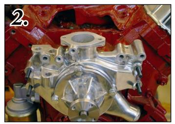
**Photo-3** Slide the Alternator Rear Support Bracket (40732-A) over the Passenger side studs and the Power Steering Rear Support Bracket (40733-A) Over The Drivers side studs Retain the Two rear supports with the four provided  $\frac{3}{8}$  x 2" Stainless Threaded Studs (S771)as shown.
