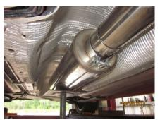
4. Install the **Muffler** onto the **Extension Pipe**. Place a **3" Band Clamp** over the **Muffler** outlet. It is necessary to support the **Muffler**. **Refer to Figure 8.**
