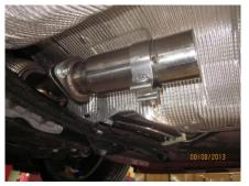
3. Install the Extension Pipe, Gasket, and Hardware onto the factory down pipe. The Extension Pipe has an angle built into it. Ensure that the pipe is angled towards the passenger side of the vehicle. Place a 3" Band Clamp over the Extension Pipe.
