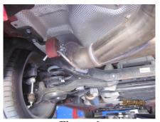
2. Place a **3" Band Clamp** over the **Tail Pipe** inlet. Slip the **Tail Pipe** inlet onto the rear of the **Over Axle Pipe**. Install the hangers into the factory isolators. **Do not tighten ANY clamps** until all parts are in place and aligned. **Refer to Figure 6.**
