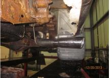
7. Align the exhaust as required. Starting at the front of the exhaust, tighten all clamps, hangers and connections. Ensure each joint is secure. Do not over tighten the Muffler Hanger Clamp; it only needs to be tight enough to prevent it from rattling.
