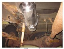
3. Install the **Muffler Hanger Clamp** over the **Muffler** and into the factory rubber insulators. Place a 3" Clamp over the Muffler outlet. Refer to Figure 5.
