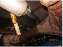
4. Insert the **Tail Pipe** over the rear axle and into the **Muffler** outlet. Refer to Figure 6.
