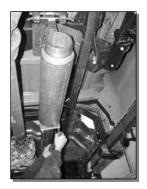
Install the Muffler over the Extension Pipe. The Hanger Clamp is used at the connection between the Muffler and the Extension Pipe and installed into the OEM rubber hanger at this position. Install the "T" Hanger Clamp into the two OEM rubber hangers located above the outlet of the Muffler. See Figure 3.
