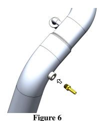
6. Insert the top end of the LHS Lower Intercooler Pipe into the 2.25" to 2.5" Hose Coupler with a 2.5" Hose Clamp (Refer to Figure 3), and the bottom end into the 2.5" X 4" Hump Hose Coupler with another 2.5" Hose Clamp. Do not fully tighten the clamps yet.
