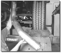
6. Install the **Tail Pipe** from the rear of the truck, over the axle and attach to the **Muffler Outlet**. Install the tail pipe hanger into the OEM hanger, adjust for best axle clearance and Tail Pipe exit location to complete. Refer to Figure 8.
