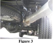
Remove the tail section from the vehicle. Refer to Figures 1 & 3.
