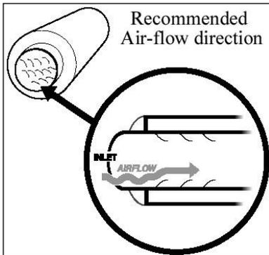
3. Install the **Muffler** over the **Extension Pipe** so that the exhaust will flow smoothly over the louvers. Refer to the illustration on the left.
